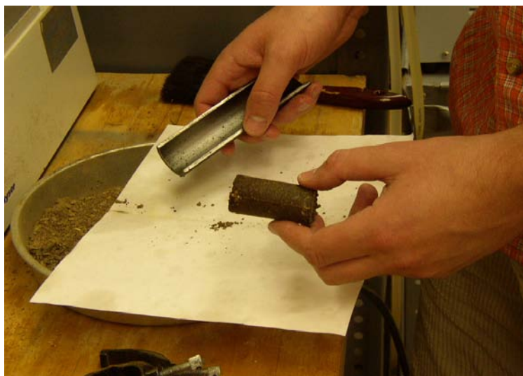
Fig. 1. Example of cylindrical compact produced from poultry litter
